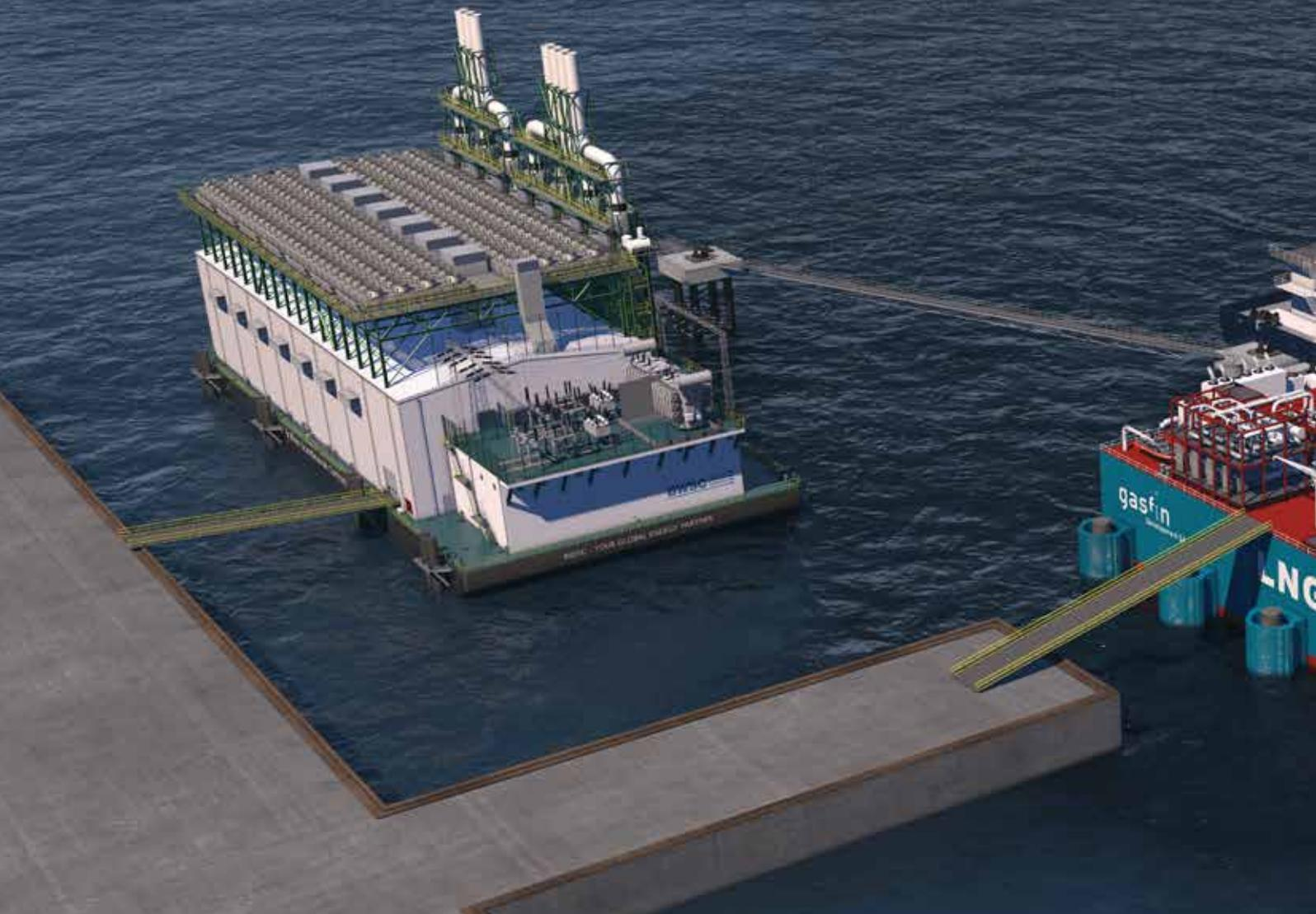
Combining small to mid-scale LNG Floating Storage and Regasification Units (FSRU) with floating power barges provides flexible and easy access to emerging energy markets.
