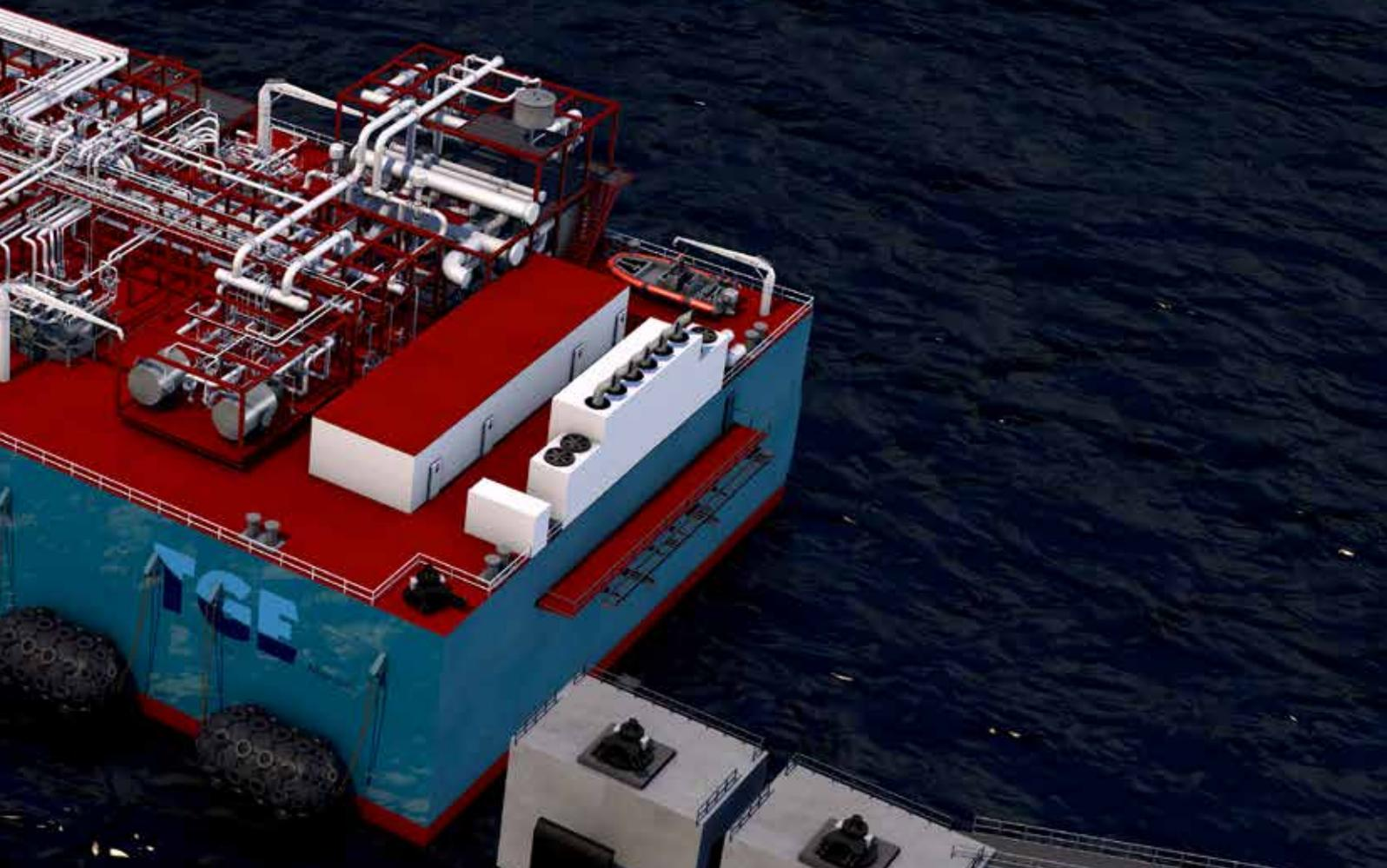
In addition to the storage system and re-gasification plant, TGE Marine takes care of the complete hull design, the design of the gas-handling system and all gas and safety-related utilities as well as electrical and control systems. The construction of the FRSU barge can be carried out by any experienced shipyard, with TGE Marine's supervision and support. During the lifetime of the project, TGE Marine will perform all after-sales services as well as necessary training of the operators.
