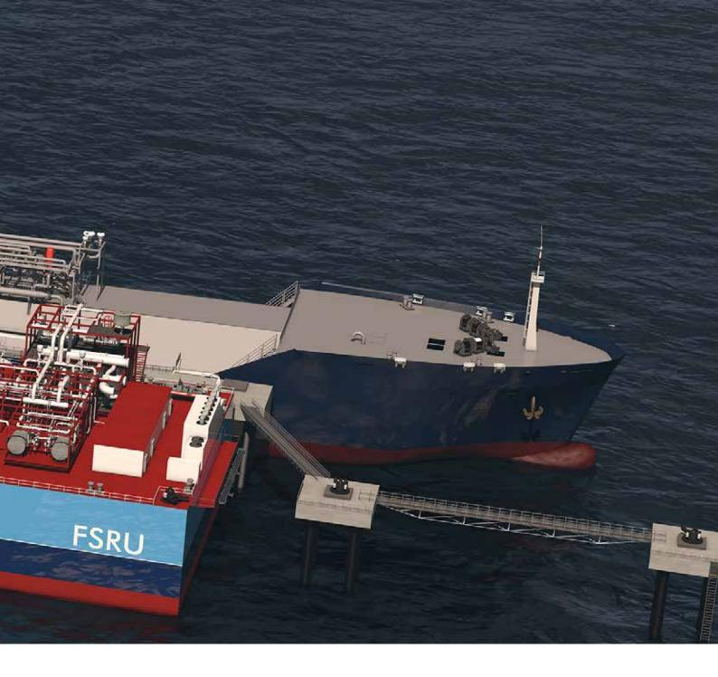
In addition to the storage system and re-gasification plant, TGE Marine takes care of the complete hull design, the design of the gas-handling system and all gas and safety-related utilities as well as electrical and control systems. With TGE Marine's supervision and support, the construction of the FRSU barge can be carried out by any experienced shipyard.
