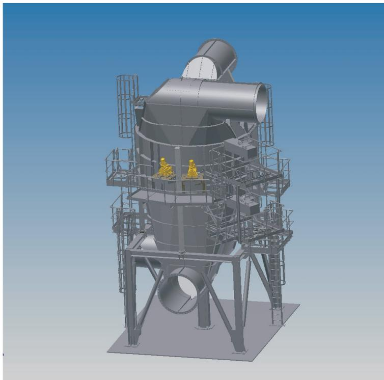
The APH is installed in the air/flue gas duct system and is used to preheat the combustion air prior to entering the boiler by exchanging heat with the hot flue gases.
