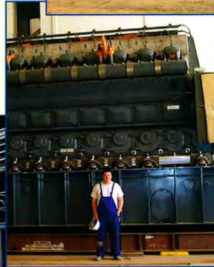
Engine on foundation
