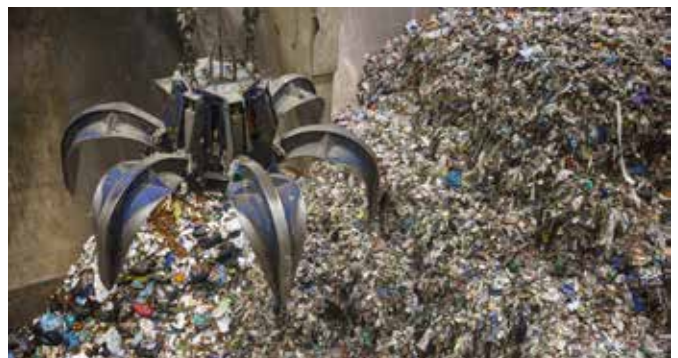
The crane will move 25 tons of waste per hour
