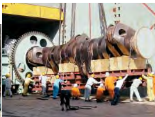
Crankshaft for Engine No. 1 for Atherinolakkos.
